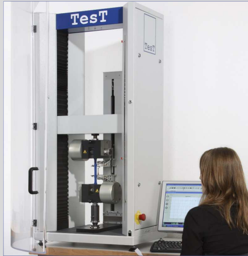
Universal Testing Machine for tension, compression and bending tests (Model 112)
