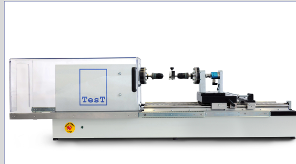
Torsion and bending tests at screws and tools for medical and dental applications
