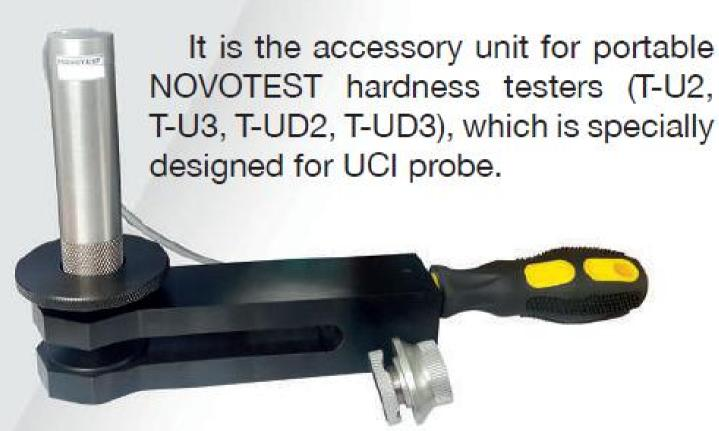
UCI Probe Test Stand NOVOTEST is used for fixation of small, thin products (even less 1 mm) during tests. It makes testing more accurate and more convenient for users.
