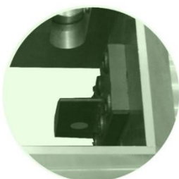
Striker knife with load cell inside
