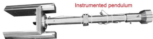
Striker knife with load cell inside
