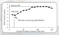
The above graph represents an example result of an annular ring inspection with the MAXWELL PECT, showing severe wall loss close to the tank shell. The corroded area extends over a length of about 80mm (3.15ins) in this case.
