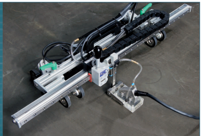
Phased Array data collected using the Swipe scanner with a 64 element PA probe
